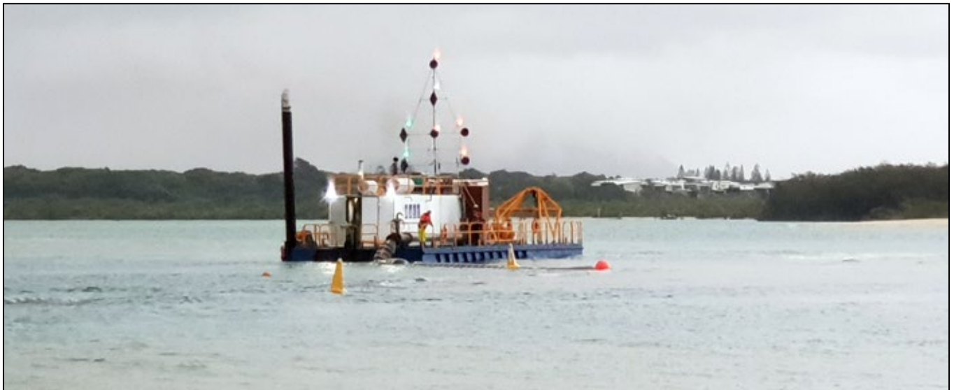
The sand-dredger barge positioned off the end of the sand spit at Cotton Tree beach.
